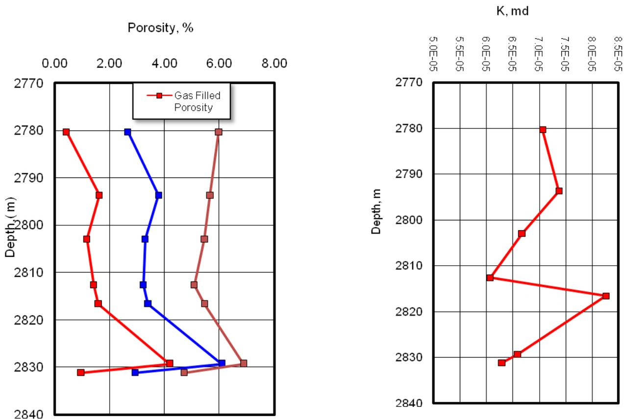
**Figure 1: Gas Filled Porosity vs. depth and permeability vs. depth for a section of the well**
